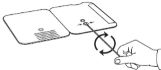
STEP 4. Peel off adhesive liner from the right edge of the test card. Close and securely seal the card. Read result in the window 15 minutes after closing the card. In order to ensure proper test performance, it is important to read the result promptly at 15 minutes, and not before. Results should not be read after 30 minutes.
